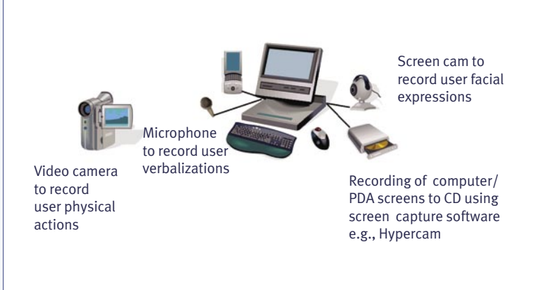
Figure 2. Basic equipment needed for conducting portable usability tests
